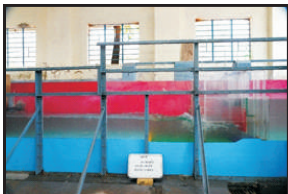
Flow condition in the Stilling Basin
