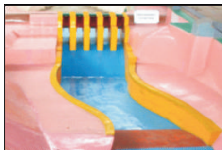
Flow conditions downstream of Spillway for Q = 6,900 m 3 /s (Gated flow) (without divide walls)
