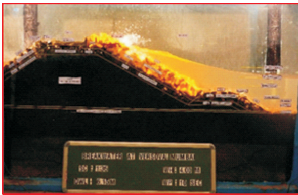
Wave flume studies at -3.0 m bed level, 8 t tetrapods in armour layer under an action of 4.0 m wave height (T= 10 sec), DWL of +6.15 m.
